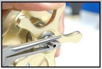
With the click pin held in place by the star drag washer, spin the star drag onto drive shaft. Use pliers to hold the shaft from spinning. 2
