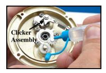
Check left side plate spool bearing for rust or wear. Oil bearing and idle gear. Apply a light coat of grease to clicker assembly to pre-
