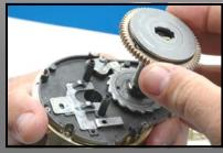
Remove drive gear, drag washers, pinion gear, yoke, yoke springs.
