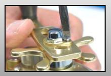
Use a small Phillips or flathead screwdriver to remove handle as-
