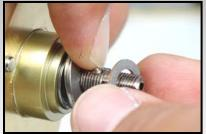
To reinstall click pin, push click pin down and use the star drag washer to hold the click pin in place.
