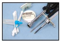
Tools and cleaning materials recommended to service reel. Some Shimano® reels come with Bantam<sup>TM</sup> Oil. These simple tools are readily available at hardware stores.
