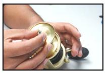
Reinstall spool and side plate. General maintenance is now complete. For further maintenance on reels that have had extensive usage, or excessive exposure to saltwater, please refer to the next page.
