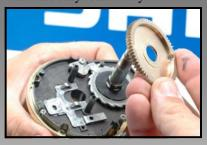
Reinstall drag washers and drive gear.
