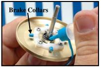
Oil spool bearing and brake collars. **Note:** Do not grease spool shaft, as it will affect freespool adversely.
