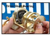
Remove spool assembly. Use Shimano® Bantam<sup>TM</sup> Oil to lubricate drive shaft bearing or bushing.
